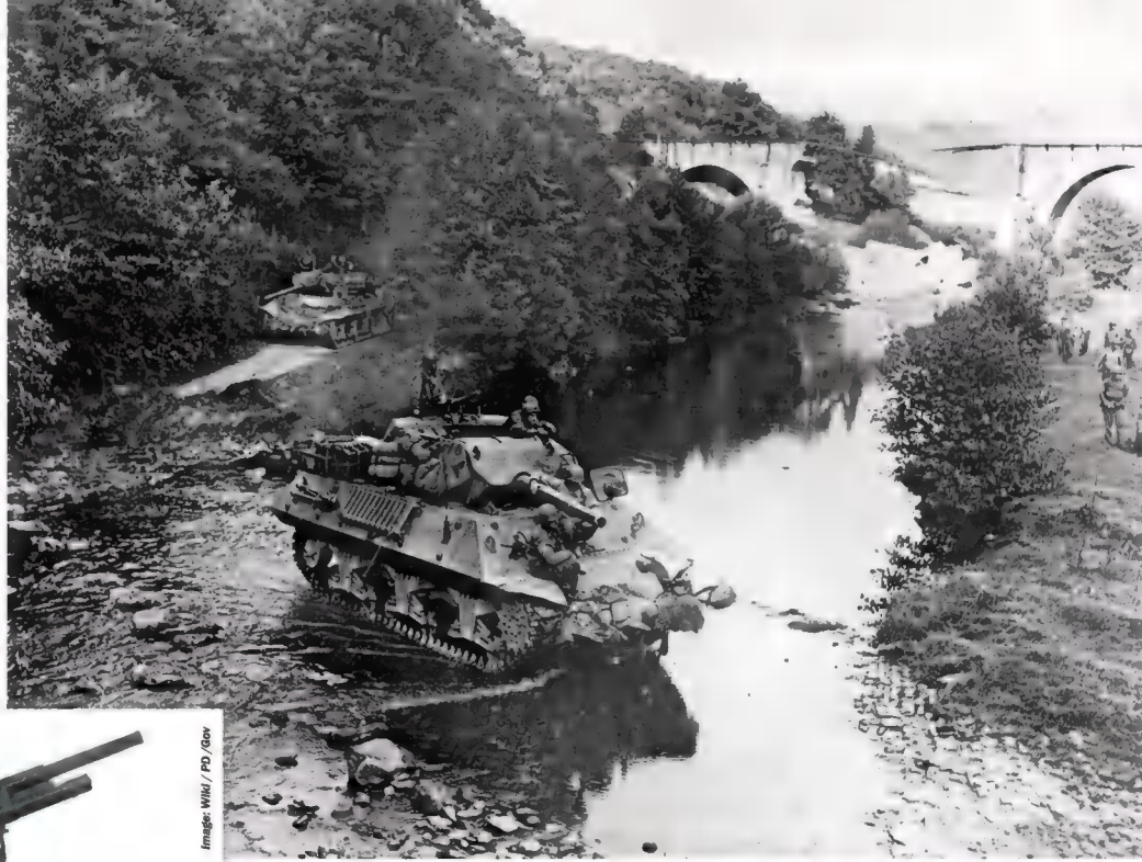
Above: The three-inch main weapons prominently visible on M10 tank destroyers prepared to cross a stream in Belgium
